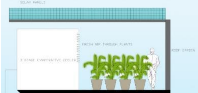
Growing our Indoor Fresh-Air. Up to 17% reduction in cooling load
