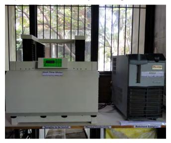
specimen thickness, and temperature difference across the specimen. Materials tested range from polyurethane foam, insulating industrial material, EPS, XPS, Glasswool and Rockwool. Specimens sized 600mm x 600 mm and of thicknesses up to 200 mm are characterized for the thermal conductivity range from 0.01 to W/m.K to 0.2 W/m.K.
